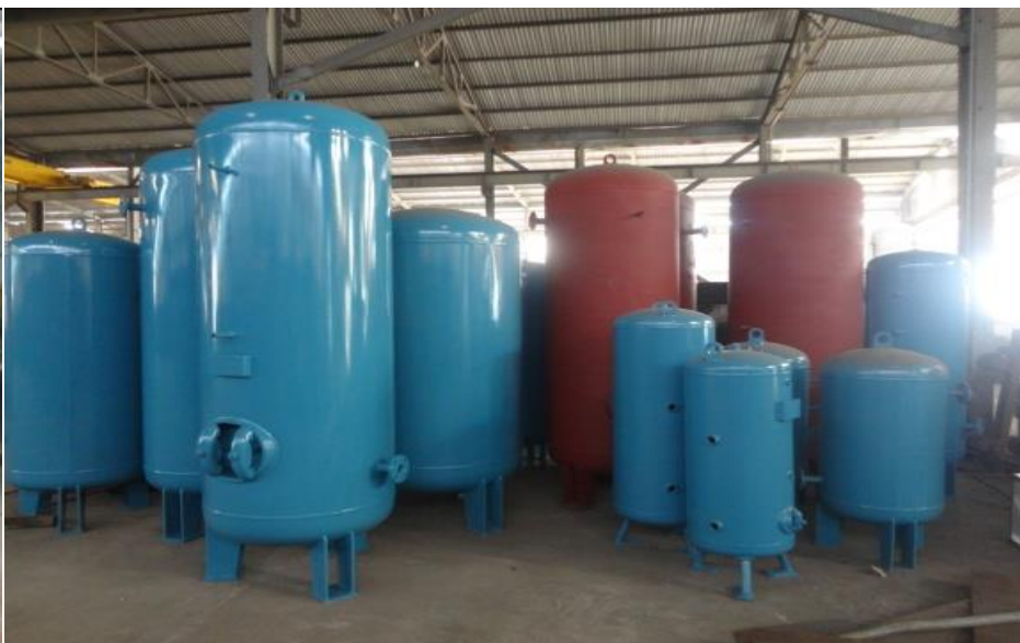
PIPE-WELDING LOCK WITH RADIOGRAPH, SURFACE HANDLED BY SAND BLAST AND SHOT BLAST...PRESSURE TEST...
